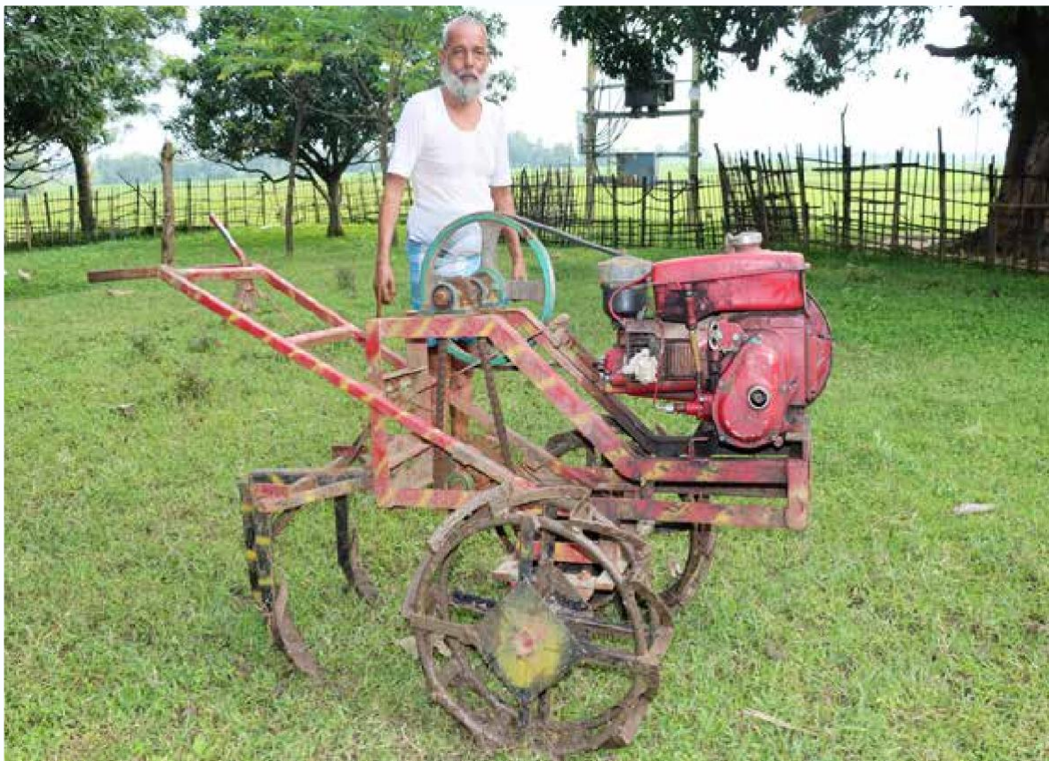
Low-cost power-tiller-cum-zero tillage machine
