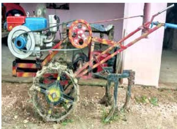
Glimpses of low -cost power tiller-cum-zero tillage machine
